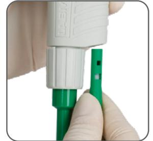
Adjustable ejector height system – to accommodate all brands of tips
