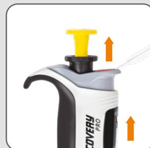
Lock the volume setting knob. Remove the red cap using the calibration key. Set the calibration switch in its upper "CAL" position.
