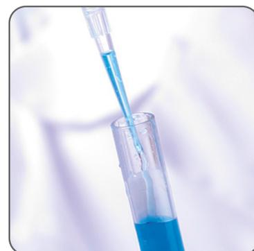
**6 Hold the pipettor vertically when aspirating the liquid**
