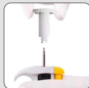
Insert the calibration key into the calibration knob. The calibration key is supplied with the pipettor.
