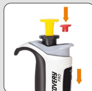
Remove the calibration key and set the calibration switch in its lower position. Place the cap on the ejector button.
