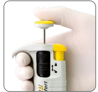
**7 Immerse the tip into the liquid correctly**
