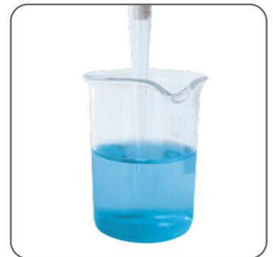
**8 Operate the pipetting button slowly and smoothly. After aspirating, wait 1 second before removing the tip from the liquid**
