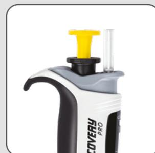
Insert the calibration key into the ejector orifice. Turn the key so as the volume indicated by the counter is equal to the average calculated volume. Refer to the user manual for details.
