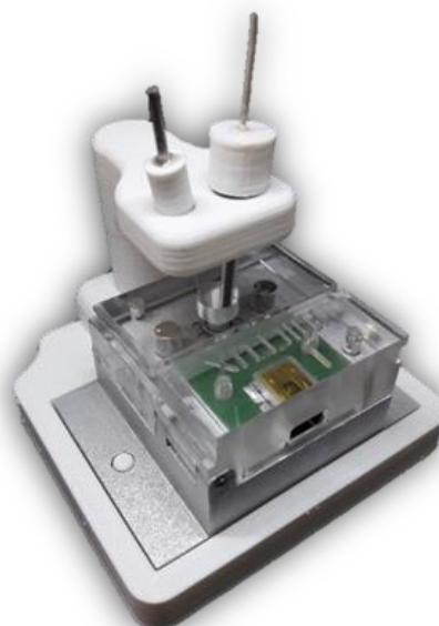
Platform with external reference & auxiliary electrodes
